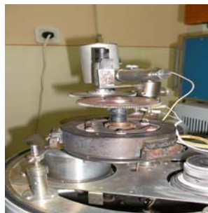
Fig.3.8. Heating and rotating system of the sample holder
